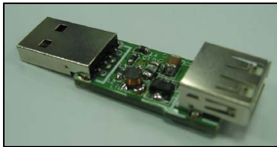
Figure-3: USB 5V-to-6.5V Port Converter
